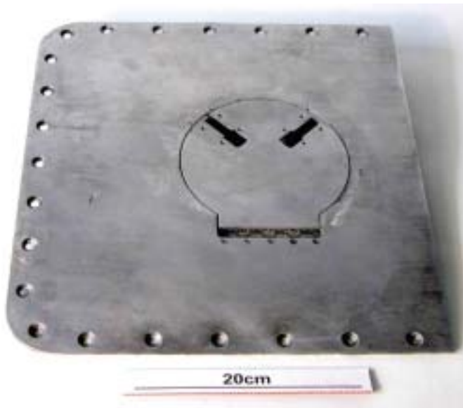
Fig. 3 Outer surface of wing panel and door after paint stripping and removal of catches.
