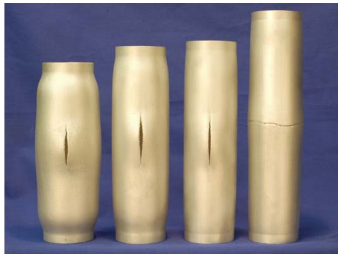
Figure 9. A set of failed test specimens tested at different biaxiality ratios: from left to right a = -0.2, 0, 0.75, 1.0 .
